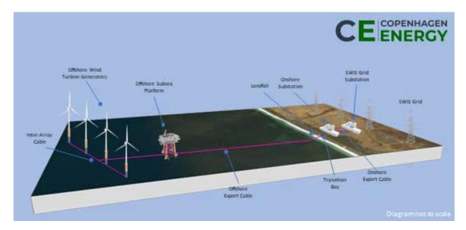
Figure 1 - Conceptual diagram showing the proposed onshore and offshore components
